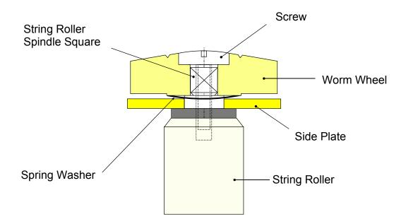
When assembling the tuner, ensure that the Spring washer is located around the diameter of the string roller spindle and that the worm wheel is seated correctly on the spindle flange. See Below. String roller should not wobble loosely.
